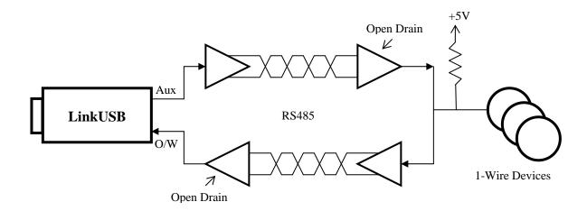
The LinkUSB™ also has a mode in which the timing of the 1-Wire waveforms is slowed to accommodate the longer turn-around times of extended host connections like that shown above. In the normal mode, network lengths of up to 3000 feet can be used (depending on the medium). In the extended mode, network lengths of between 2000 and 6000 feet can be achieved.
