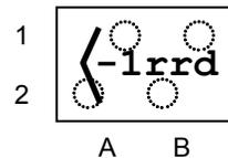
Flip Chip, Top View with Laser Mark, Contacts Not Visible.
