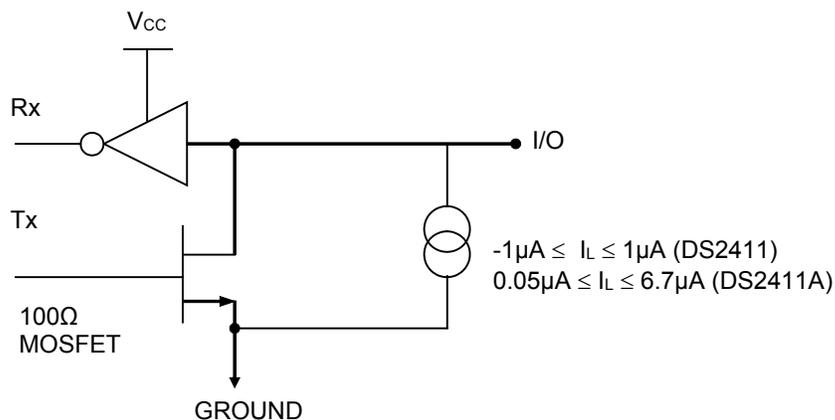
**Figure 4. BUS MASTER CIRCUIT**
