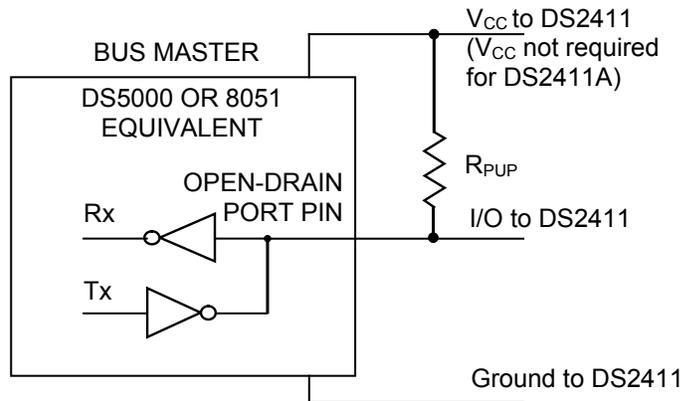
$R_{PUP}$  must be between 0.3 k $\Omega$  and 2.2 k $\Omega$ . The optimal value depends on the 1-Wire communication speed and the bus load characteristics.
