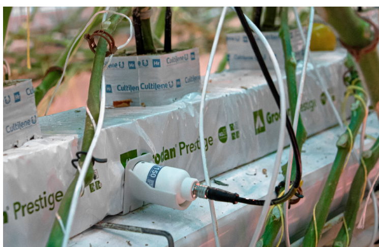
Figure 5: WET150 sensor with a plastic sensor stand
