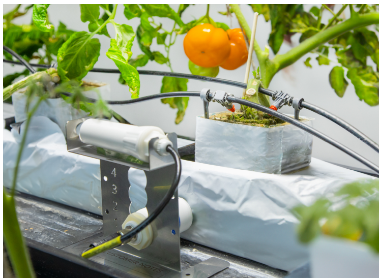
Figure 4: WET150 sensor with an installation bracket
